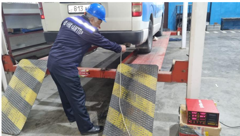
The process of measuring exhaust gases for the content of CO and CH on the gas analyzer
