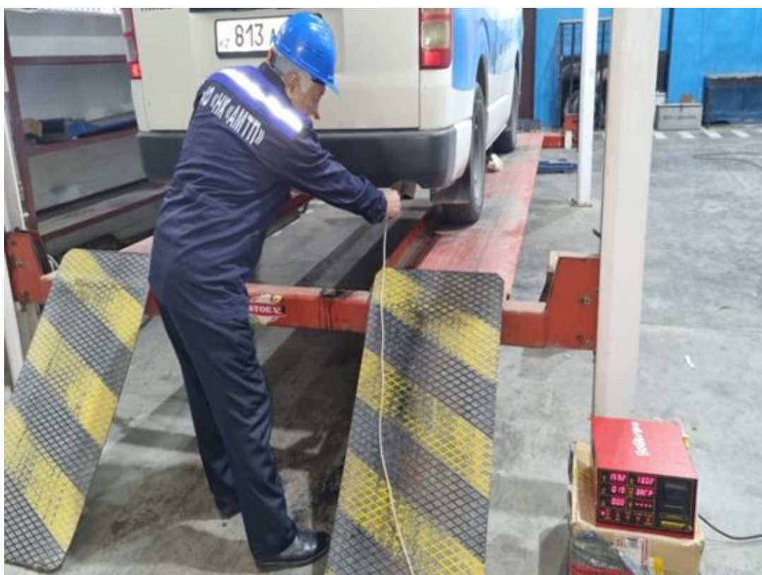
The process of measuring exhaust gases for CO and CH content using a gas analyzer
